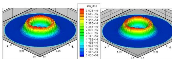
Fig. 8. Cycle-averaged distributions of number densities of electrons (left) and ions (right) for a RF magnetron argon plasma.
