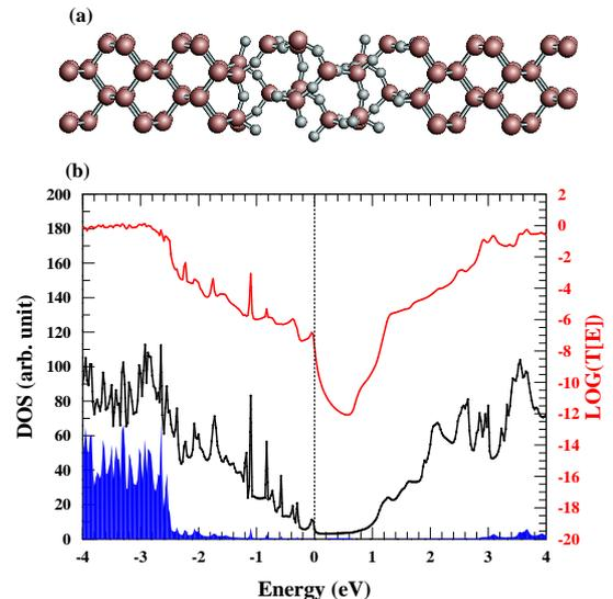
Fig. 2. (a) Atomic structure of the oxide device, where  $\alpha$ -quartz  $\text{SiO}_2$  is sandwiched between two Si(100) electrodes, and (b) the total transmission (upper curve) and the density of states (lower curve). The shaded area represents the DOS projected onto the oxide region.
