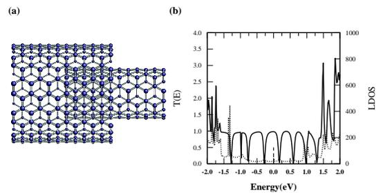
Fig. 1. (a) Atomic structure of the (5,5)/(10,10) telescoping carbon nanotube and (b) the calculated total transmission (solid line) and the local density of states (dotted line).
