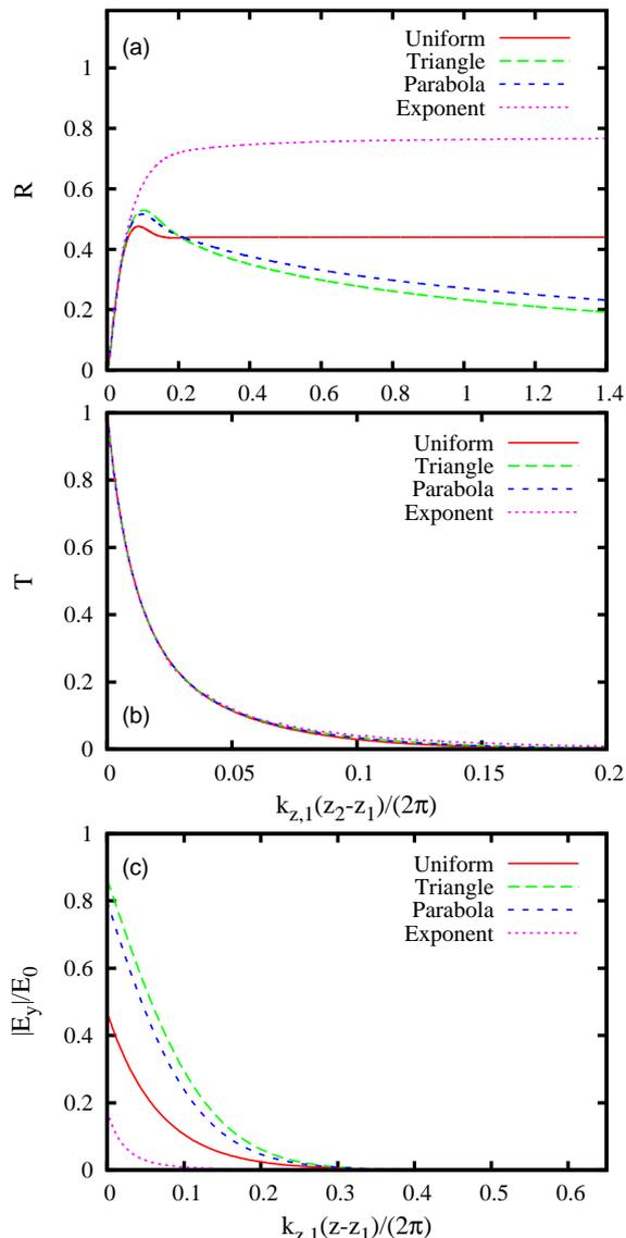
Fig. 4. (a) Reflectance, (b) transmittance, and (c) electric field distribution (at  $k_{x,m}x = \pi/2$  and with  $z_2 - z_1 = 0.1$  m) for  $TE_{m,0}$  wave under argon gas of 1 atm in a rectangular waveguide.  $w/2\pi = 2.85$  GHz,  $k_1 = k_{gas} = k_3 = w/c$ ,  $\gamma_{m,0}^2 = 1.9 \cdot 10^3 \text{ m}^{-2}$ , and  $n_{e,ave} = 7.9 \cdot 10^{19} \text{ m}^{-3}$ .
