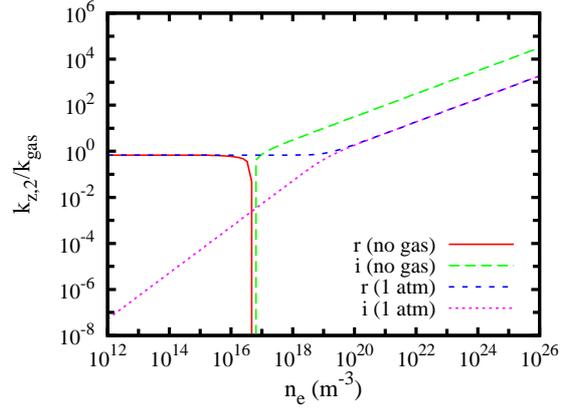
Fig. 1. Real ( $r$ ) and imaginary ( $i$ ) parts of  $k_{z,2}/k_{gas}$  as a function of the electron density in a rectangular waveguide without any background gas and with argon gas of 1 atm.  $w/2\pi = 2.85$  GHz and  $\gamma_{m,n}/k_{gas} = 0.73$ .
