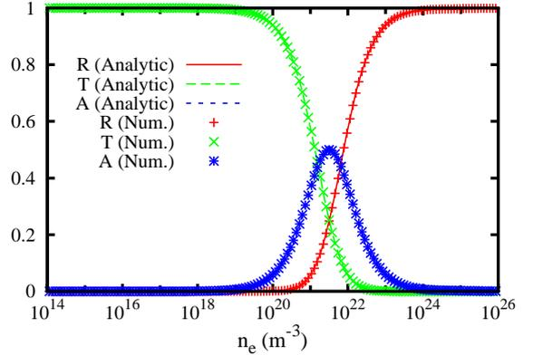
Fig. 2. Reflectance (R), transmittance (T), and absorbance (A) as a function of the uniform electron density under argon gas of 1 atm in a rectangular waveguide.  $w/2\pi = 2.85$  GHz,  $z_2 - z_1 = 100 \mu\text{m}$ ,  $k_1 = k_{gas} = k_3 = w/c$ , and  $\gamma_{m,0}^2 = 1.9 \cdot 10^3 \text{ m}^{-2}$ .
