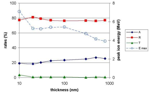
Fig. 3. Variations of maximum proton energy and laser absorption (A), reflection (R) and transmission (R) rates with thickness of a  $150n_c$  target. The  $0.8 \mu\text{m}$ -wavelength laser pulse is incident at  $30^\circ$  from target normal, has a 30 fs FWHM duration and a peak intensity of  $10^{19}$  W/cm<sup>2</sup>
