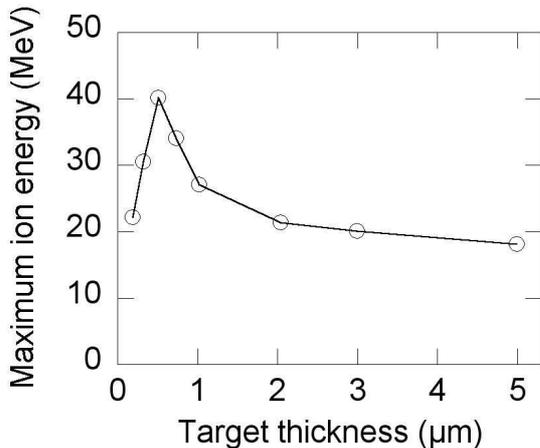
Fig. 2. Variations of peak proton energy with thickness of a  $10n_c$  target. The normally incident laser pulse has a 36 fs FWHM duration and a peak intensity of  $10^{20}$  W/cm<sup>2</sup>
