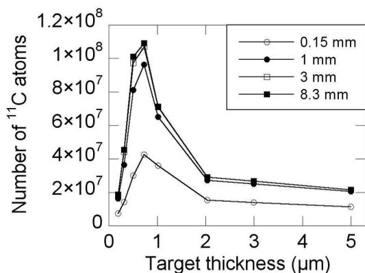
Fig. 4. Number of  $^{11}\text{C}$  atoms produced by  $^{11}\text{B}(p,n)^{11}\text{C}$  reaction in a solid boron catcher of variable thickness, as a function of the proton-producing target thickness
