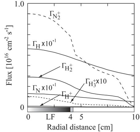
Fig. 5. Arrival flux of ions and radicals at biased organic low-k surface and earthed metallic plate. External conditions are 50 mTorr in  $N_2/H_2(50\%)$  and 100 MHz and 300 V (plasma source) and 1 MHz and 700 V (bias source).
