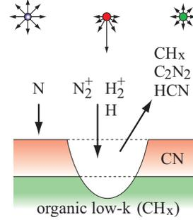
Fig. 4. Surface model of etching of organic low-k materials by  $H_2/N_2$  plasma.
