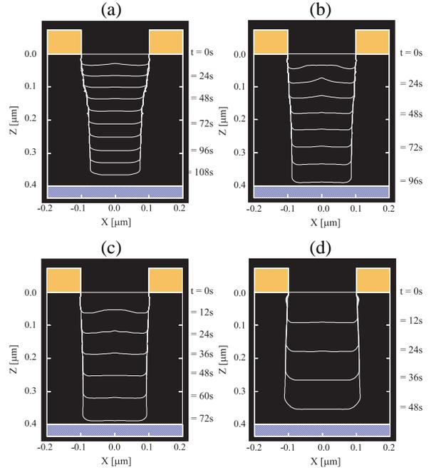
Fig. 7. Feature etching profile of organic low-k (FLARE) as a function of gas mixture.  $N_2/H_2(5\%)$  (a),  $N_2/H_2(25\%)$  (b),  $N_2/H_2(50\%)$  (c), and  $N_2/H_2(75\%)$  (d). Other external conditions are in the text.
