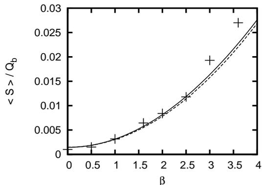
Fig. 3. Normalized collisionless heating power as a function of  $\beta \equiv \tilde{J}_h/\tilde{J}_l$ , with  $\tilde{J}_h$  as the parameter varied (so that  $H_l$  is constant) and with  $\alpha = \omega_h/\omega_l = 13$ .
