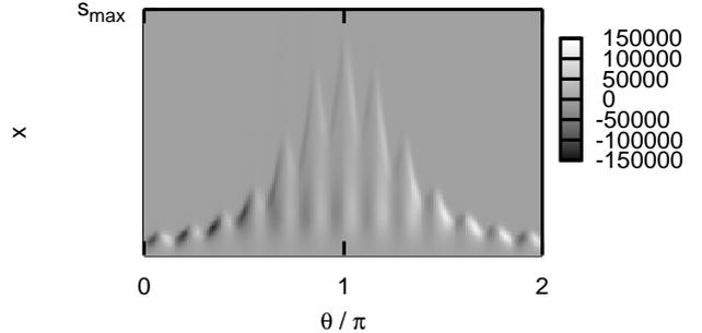
Fig. 1. Collisionless heating power as a function of space and time, calculated by the particle simulation, with  $\tilde{J}_l = 10 \text{ A m}^{-2}$ ,  $\omega_l = 2\pi \times 2 \text{ MHz}$ ,  $\tilde{J}_h = 20 \text{ A m}^{-2}$  and  $\omega_h = 2\pi \times 26 \text{ MHz}$ , and the plasma parameters discussed in the text. The ion sheath edge is at  $x = 0$  and the electrode is at  $x = s_{\max}$ .
