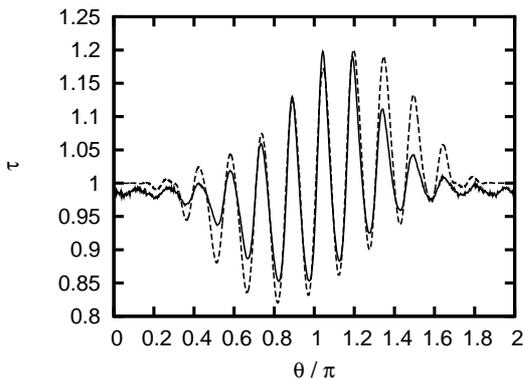
Fig. 2. Temperature of electrons in the sheath computed from the analytic theory of the text (solid line) and from the particle-in-cell simulation (dashed line), for the conditions noted in fig. 1.
