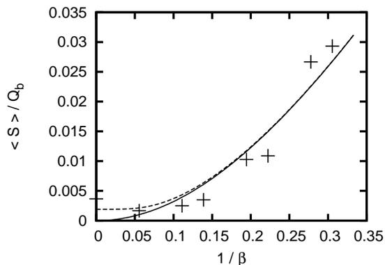
Fig. 5. Time averaged electron heating power as a function of  $1/\beta \equiv J_l/J_h$ , where the parameter varied is the low frequency current density  $J_l$ . Other parameters held constant are the high frequency current density  $J_h = 36 \text{ A m}^{-2}$ , and the two frequencies  $\omega_l = 2\pi \times 2 \text{ MHz}$  and  $\omega_h = 2\pi \times 26 \text{ MHz}$ .
