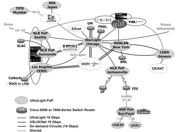
Fig. 2. The UltraLight network testbed as of August 2006
