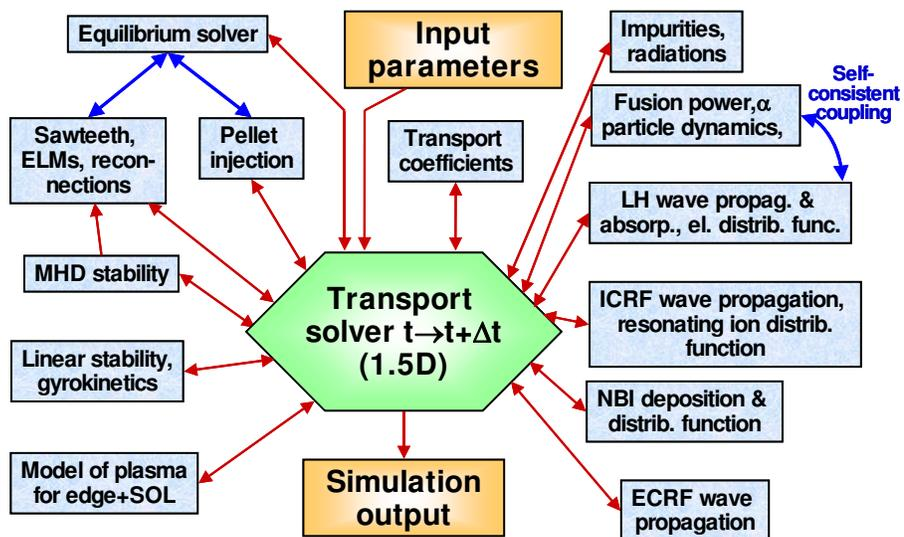
Fig. 2. Schematic structure of a tokamak simulator
